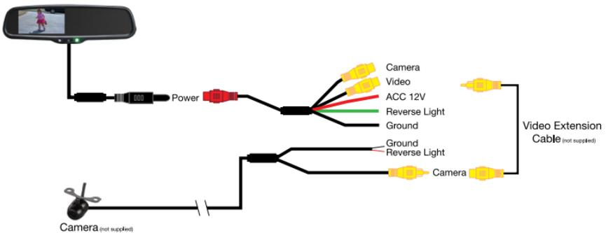
Connect the Rear View Mirror Monitor to the supplied harness and the supplied harness to the wiring of the car as instructed in the below image:
