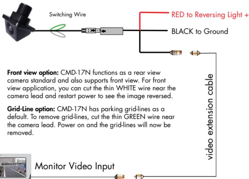
**Front view option:** CMD-17N functions as a rear view camera standard and also supports front view. For front view application, you can cut the thin WHITE wire near the camera lead and restart power to see the image reversed.
